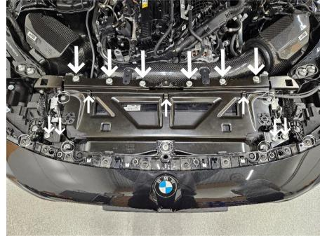
Remove the 4 plastic retaining clips from the top of the bumper cover.
