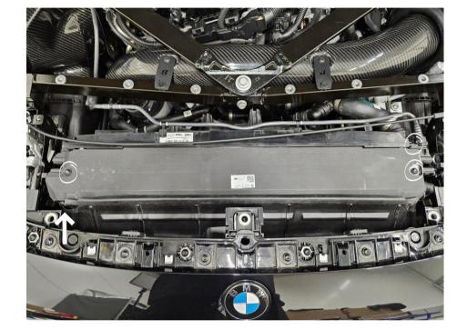
Gently pull the upper part of the bumper cover forward and remove the four plastic clips holding the plate to the front air duct. The ones on the left side is shown in picture.
