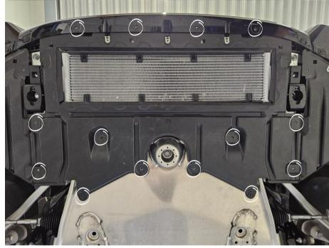
Remove the lower lip by loosening 11x 10mm hex screws and move the lip in a rearward then downward direction.
