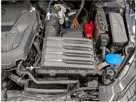
Remove the 2x T25 holding the air filter ducting and remove it.
