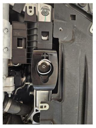
Drill out the rivet holding the curb descent damper. Then remove the damper and punch the rivet away from the hole in the impact beam. Repeat on the other side.
