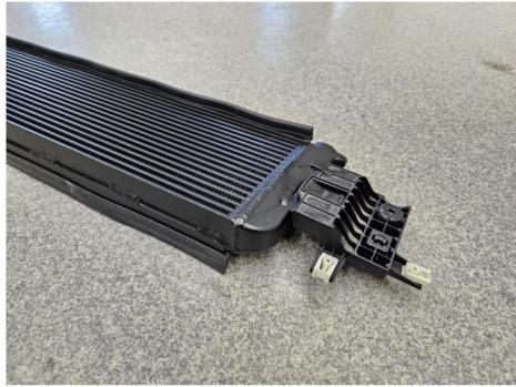
Remove the 2x 10mm hex screws holding the oil cooler brackets. Then remove the oil cooler by moving it forward, then downward.
