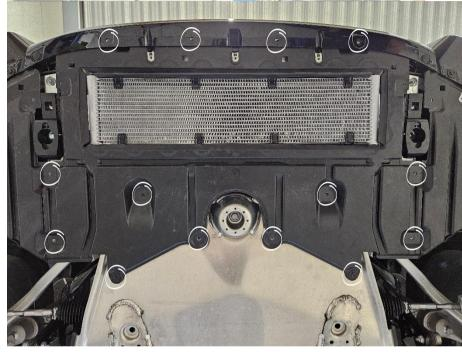
Remove the lower lip by loosening 11x 10mm hex screws and move the lip in a rearward then downward direction.
