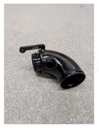
Step 5 (Only when installing do88 3" turbo inlet pipe)
