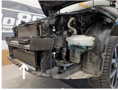
Relocate the hood support to the fender. Remove the  $2x\ T25$  holding the air filter ducting and remove it.
