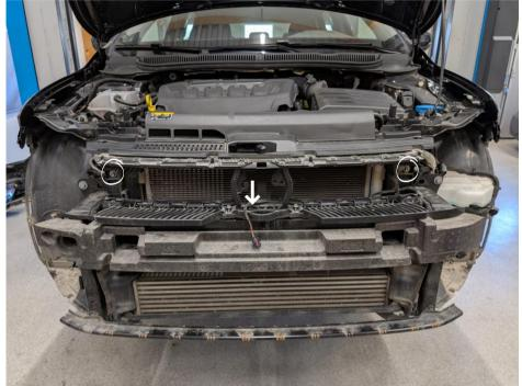
Remove the headlights by undoing 3x T30 screws on the top and 2x T25 in the fender on both sides. Then lift the front of the headlight out of it's support and disconnect the electrical connector before removing the headlights from the car.
