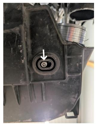
Push the cooling stack into correct position, start with the two upper radiator supports and then fixate the intercooler with the included allen 5mm screws from underneath.
