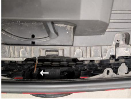
Remove the 4x T25 holding the upper part of the bumper.
