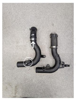
Preinstall the throttle body hose and its hose clamps and clock them as the OE hose. Transfer the sensor from the OEM pipe to the do88 pipe and secure it with the included M5x16 T25 screws.
