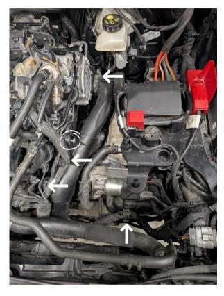
Loosen the hose clamps on the turbo outlet hose. Release the wiring harness retainers marked in picture. Undo the T30 holding the pressure pipe and then remove the pipe.
