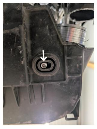
Push the cooling stack into correct position, start with the two upper radiator supports and then fixate the intercooler with the included allen 5mm screws from underneath.
