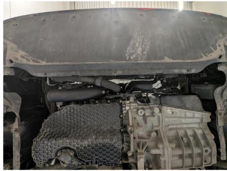
Install the pipe to the throttle body and secure its hose clamp. Then fasten both pipes to the engine.
