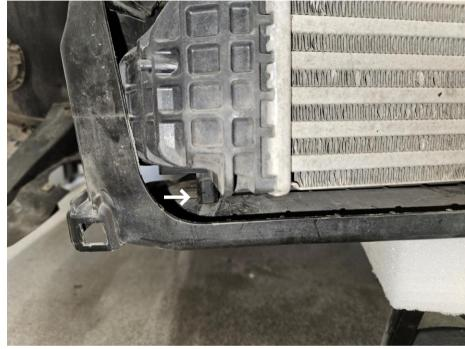
Separate the radiator support frame and the cooling stack on the left side by tilting the radiator backwards and lift the intercooler out of its lower rubber grommet.
