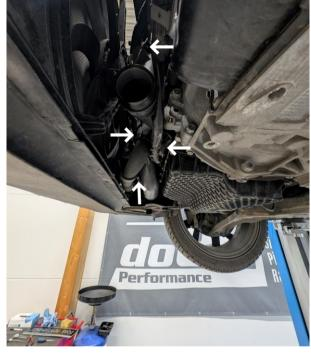
Loosen the hose clamps on both the inlet and outlet hoses of the intercooler and then remove the hoses.
